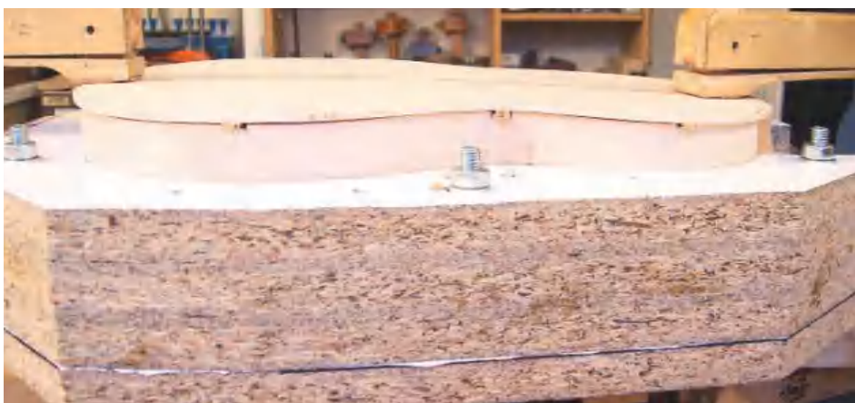
STEP 34. Locating the correct position for the back of the instrument
